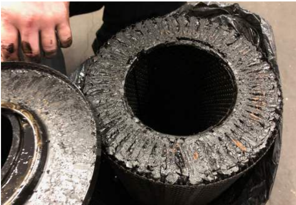
A result of non-optimised fuel blending
